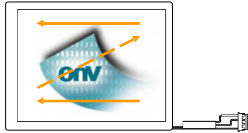
Fig. 2 Reverse scan (Pin31, DPS = High)
